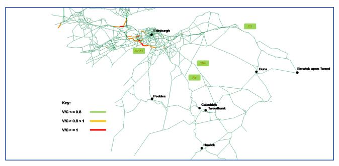
Figure 50: Volume over Capacity Ratio (V/C), 2024 Reference Case, PM Peak Hour
