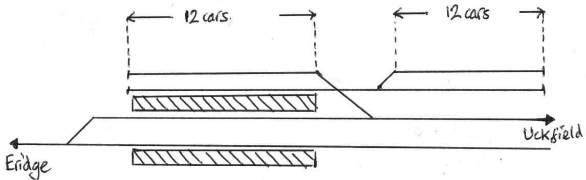
Crowborough station – proposed layout to accommodate four stabled 12 car trains in four sidings.
