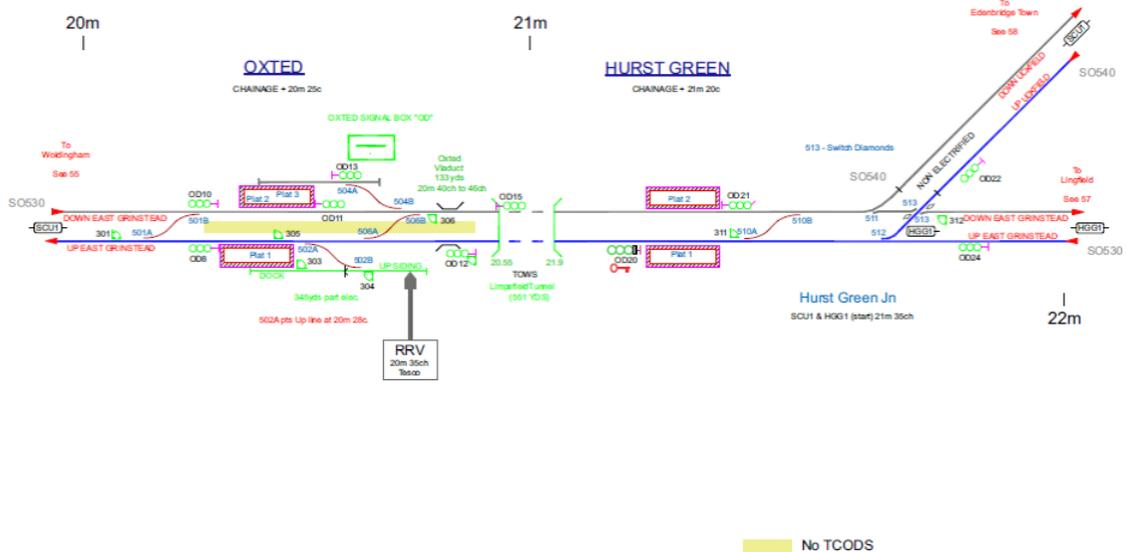
Figure 3 – Oxted / Hurst Green track and signalling layout
